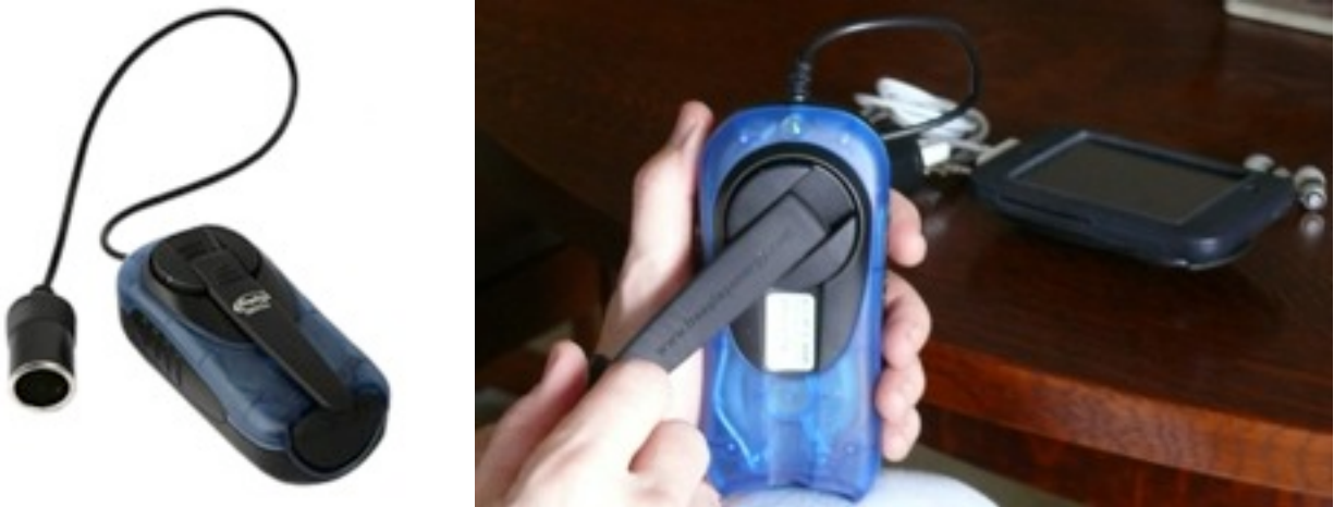
Figure 1 shows the FreeCharge 12V with the crank retracted (left) and with the crank in action (right).
